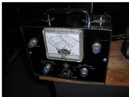
This is an ECI Courier Port-A-Lab (Dummy load, RF sniffer, SWR/Wattmeter, and Modulation Monitor)
