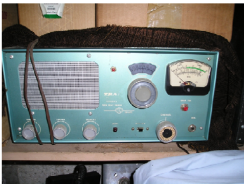
This is a Tram TR-27C about 1960 - VFO receive/23 channel crystal transmit.
