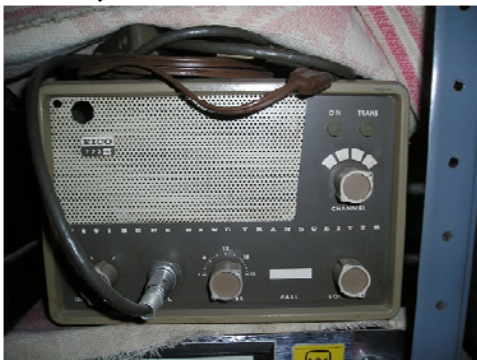
This is an EICO 772 kit about 1963 4 channel transmit w/VFO receive but a poor performer. MORE PHOTOS PG 9
