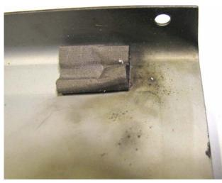
Copper trace areas vaporized by the transient flash are clearly visible. Aluminum electrolytic caps C452 and C445, on either side of the common mode choke T35 that filters the incoming 12 volt power, were physically intact but showed reduced capacitance, although leakage was about normal. One winding of T35 burned through at the point where it was soldered to a mounting pin.
