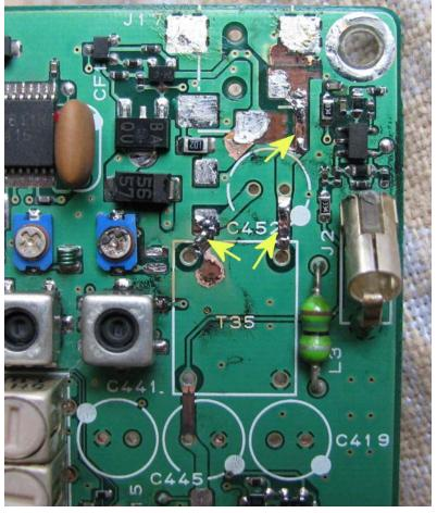
Although the blue trimmer cap shows discoloration from arc soot on the adjustment slot, it was electrically intact, as well as was the other components associated with it (430MHz band transmit filter).
