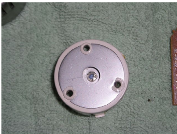
Figure 4 Americium-241 pellet in the center of the disk
