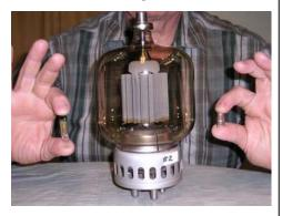
The tube on the left is a sub-miniature "pencil" tube used in portable receivers in the 1960s. These tubes, made by Raytheon, were competing with the early transistor sets. We know who won and the pencil tubes were phased out. They used very little filament and plate operating power.
