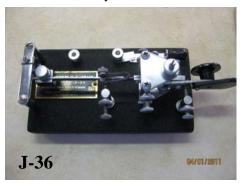
This bug is the Vibroplex J-36. The label says Signal Corps-U.S. Army. The serial number is 1673. It has a contract date of June 27, 1942. I am not sure what that means since these were manufactured from 1941-1945. It might mean that
