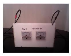
This pic is backwards but shows Voltage and Leakage Current Meters.
