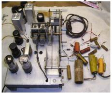
Tubes were tested with all showing good emission. The chassis and other parts were as bright and shiny as when they were new. Taking the built-in speaker off the cabinet exposed a 1 inch thick 60 year old dust mat which, when removed, displayed a perfect cone.
